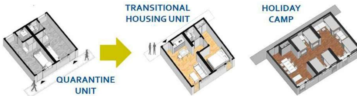
Figure 34. Transformation possible of quarantine facilities' module
