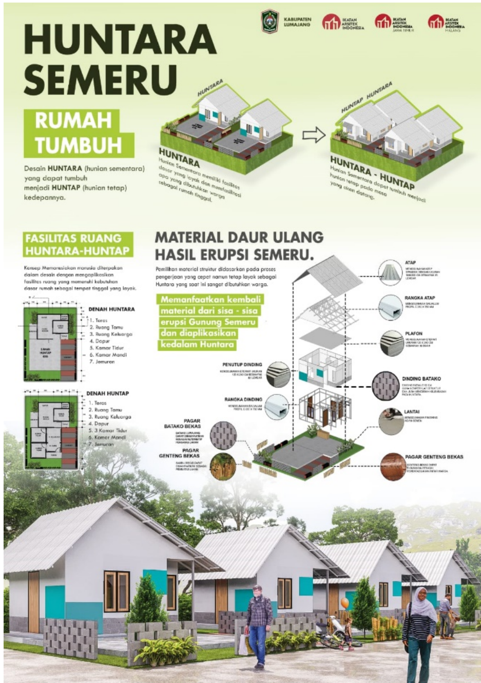
Figure 15. Design of temporary housing, based on the concept of core housing. Source: (Permana & Hidayat, 2022)
